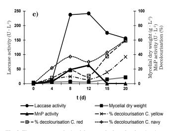
Fig. 3. Time course analysis of the growth, dyes decolourisation, laccase and MnP production by G. aff. zonatum B-18 on: a) Kimura medium, b) Kimura medium + dyes mix c) Kimura medium + dyes mix and textile additives (simulated textile effluent).
